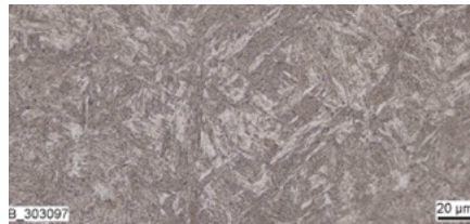
Tempered state, oil cooled 200:1
