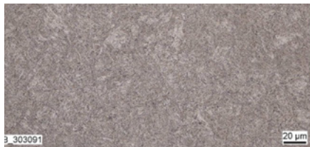
Tempered state, water cooled 200:1
