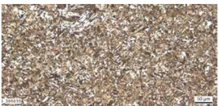
Tempered state, water cooled
