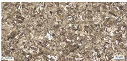
Tempered state, oil cooled
