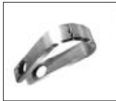
HASTELLOY B-2 alloy Annealed + 1 hr at 1290°F (700°C) (Intergranular cracking, 3 hours)
