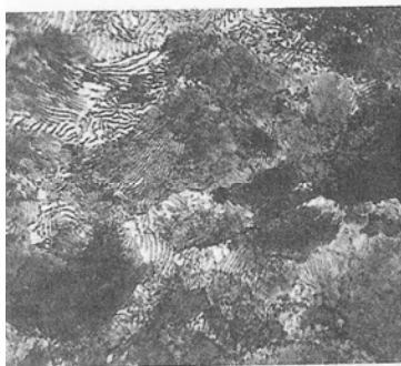
(b) Fine Lamellar Pearlite Formed at 1100°F (600°C)
