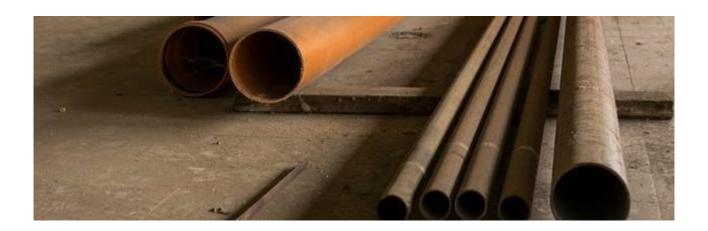
The term "random" refers to the fact that the pipe mill can control that the pipe length is between a min-max value, but cannot control the exact length of every single pipe (which will be variable, within the given range).
