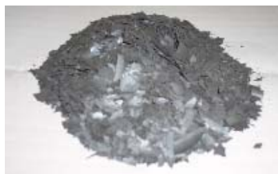
图 4 割管取出氧化皮重约 90g Fig. 4 Pipe cutting out the weight of about 90 g oxide skins
